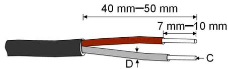
$$C = 0.5 \text{ mm}^2 - 1.0 \text{ mm}^2, D \leq 2.8 \text{ mm}$$
